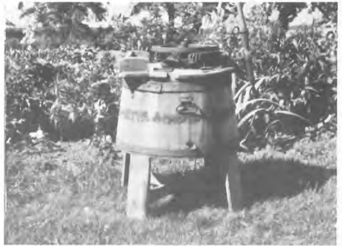
This washing machine was used by Mrs. Fred Scharbius in the early 1900's, and also by her daughter, Mrs. Arthur Utech. This early machine consisted of a paddle which worked as an agitator and was moved back and forth by the handle on the outside. The inside of the washer had a corrugated effect like a washboard.
