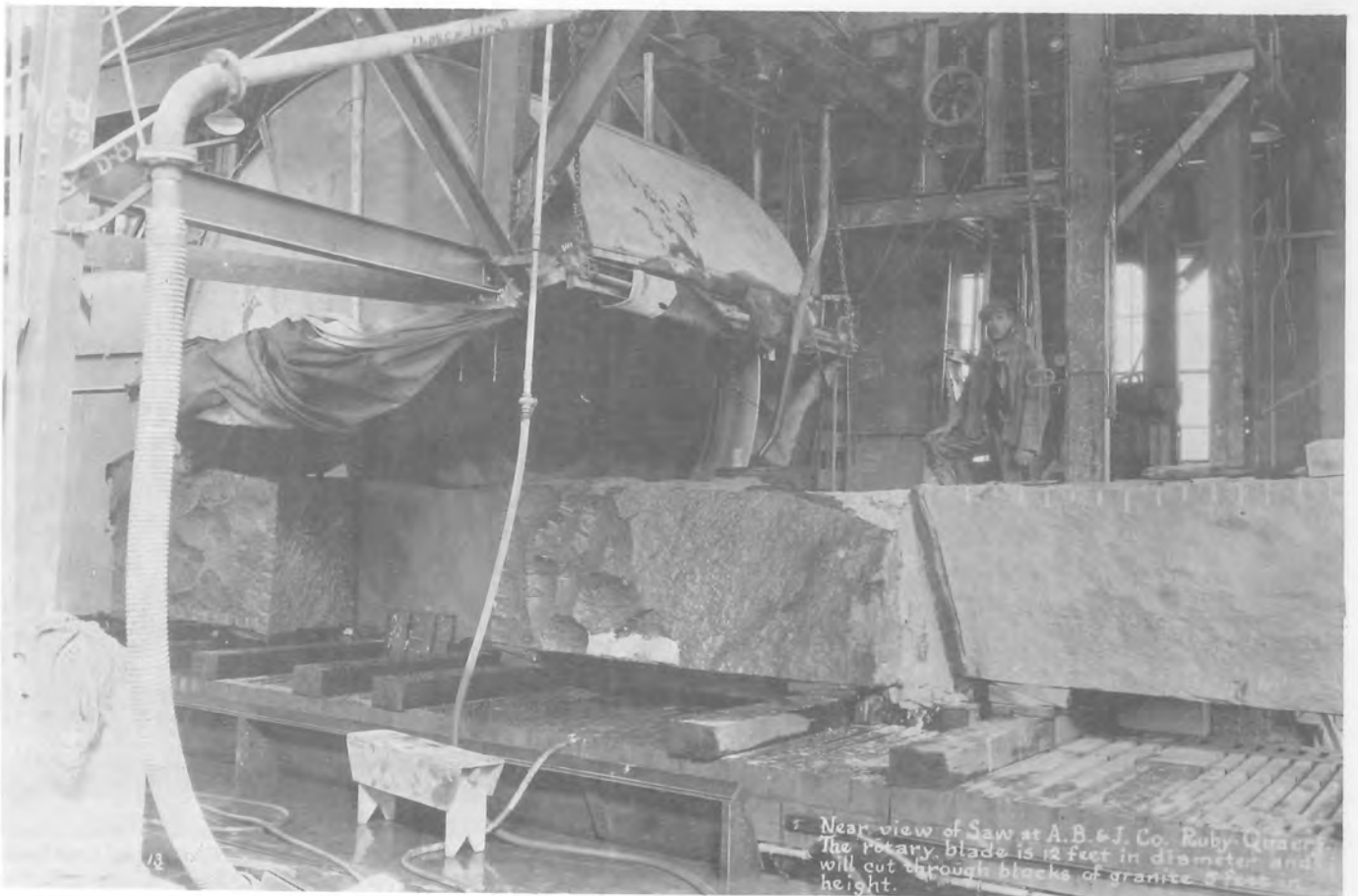
Near view of saw at A. B. & J. Co. Ruby Quarry. The rotary blade is 12 feet in diameter and will cut through blocks of granite 5 feet in height.
