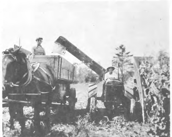
One of the first corn field choppers in this area, purchased in 1925. Clarence Utech driving the Fordson tractor and Robert Laatsch driving the team of horses to catch the chopped silage as it is delivered from the machine.
