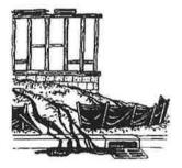
A poorly installed silt fence will not prevent soll erosion. Fabric must be buried in a trench and sections must overlap (see diagram on back of this fact sheet).
