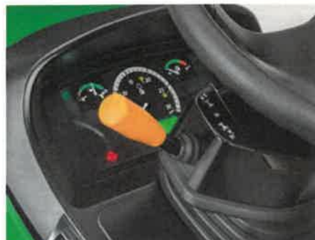
PowrReverser transmission lever
