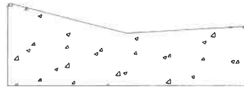
TYPE "A" MIAMI CURB & GUTTER STD. 201.1
