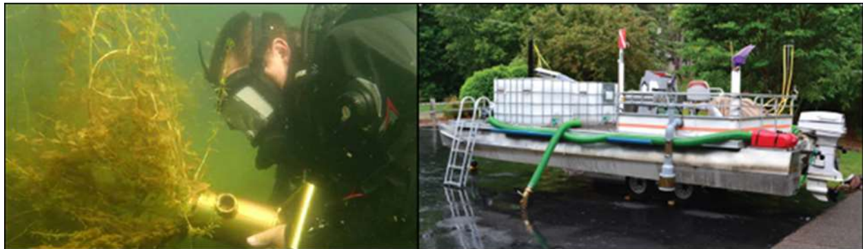
Figure 62: DASH – Feeding EWM into the underwater Suction Hose (Marinette Co.); and a sample DASH Pontoon Boat (Beaver Dam Lake Management District)
