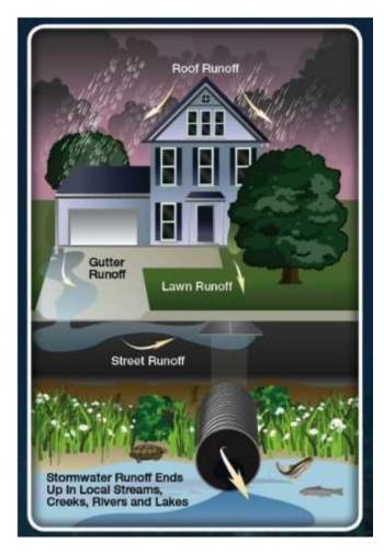
$Storm\ Water\ Runoff\ Illustration\ (\underline{http://www2.erie.gov/environment/index.php?q=how-can-you-prevent-stormwater-pollution)$
