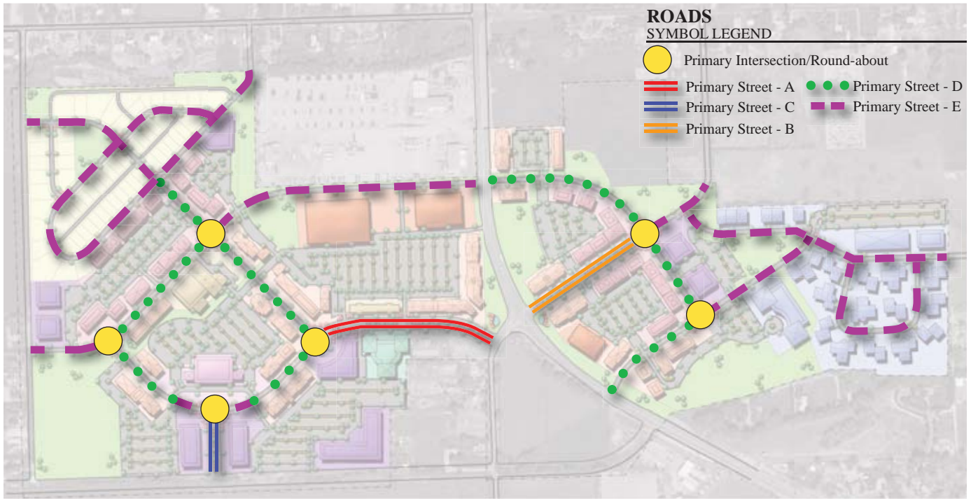
Illustration of "Primary" roads with each specific cross section referenced. Note: all roads shown are considered "Primary"
