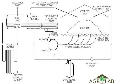
Magazine. The system's design greatly differs from Jean Pain method as it requires a significant amount of technological investment (see design below). The system has a compost load capacity ranging from 150-800 tons and captures thermal energy ranging from one to five million BTU's per day. Using vapor capturing technology, Diamond Hill reports output temperatures of 131 to 149 degrees Fahrenheit, with compost pile temperatures
