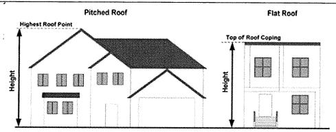
structure, excluding architectural elements such as chimneys, flag poles, skylights, etc., and draw a line parallel to the finished grade shown on the elevation plans. The building height is the vertical distance between finished grade and the highest point on the building, provided that the measured elevation does not include fill or berms.
