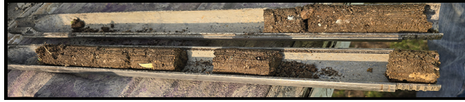
Pictured: soil core samples from below hockey rink
